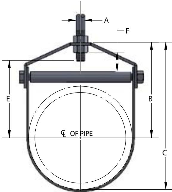
“E” dimension includes exposed rod threads beyond bottom of the hex nut. Exposed rod thread dimension is equal to the diameter of the rod used.
