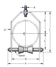
"E" Dimension includes exposed rod threads beyond bottom of hex nut. Exposed rod thread dimension is equal to the diameter of the rod used.
