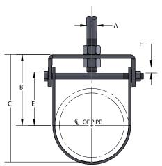
"E" Dimension includes exposed rod threads beyond bottom of hex nut. Exposed rod thread dimension is equal to the diameter of the rod used.
